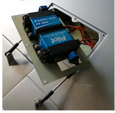
2.Place the servo over the servo plate making sure that the arm moves freely within the provided slot, and mark out the placement of the four screw holes. drill out the four holes in the plate, then securely screw the servo to the inside of the plate using the metal screws provided
