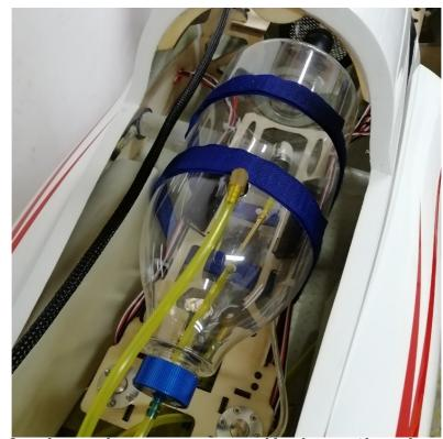
To arrange the fuel tank, connect all the oil tube (or you can connect it later), and stick the Velcro stick on the tank support frame. Also, you need stick the Velcro stick on the fuel tank, to arrange the tank on the support frame, use Velcro stick tape to
