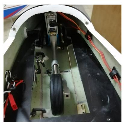
Install the nose retract gear to the fuselage.
