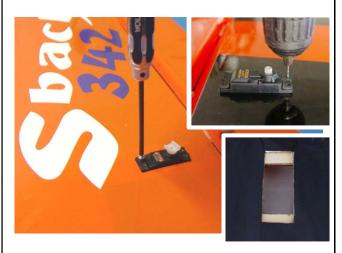
6. Install the servo arms facing toward the wing tip. Measure and cut the extra wire. Then bend to a sharp of "z" as shown .Keep the aileron panel on the neutral position
