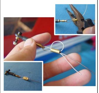
NOTICE: The coupler is best to thread half way into ball link for further tightening next 2.Mount servo with mounting screws and face the brand toward the rudder. Install the servo arm ball links with bolts and nuts.
