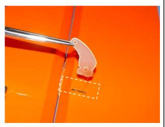
3. Slide the horns into slot slightly and wipe away excess epoxy with rubbing alcohol
