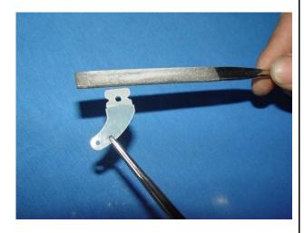
2. Cut out the cover for horns location carefully. Apply the 30 minutes epoxy inside the pre-cut slot, and coat the horn with epoxy
