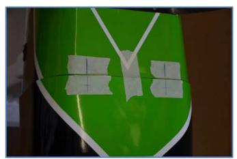
The cowling is installed with a single pre-installed bolt on the top half, from the inside of the fuselage going forwards, and two additional bolts going through the cowling from the bottom.
