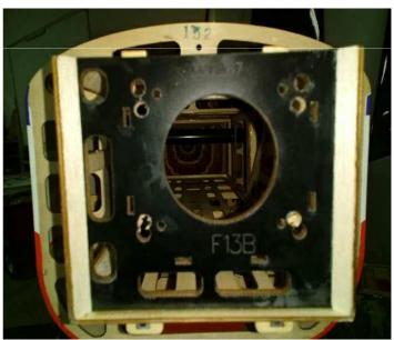
For easy installing the engine, it is recommended to trace the fixing points for your engine, and use this to mark the locations to drill and later fix the engine.
