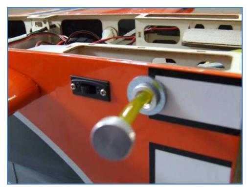
Locate the appropirate hole and install the fuel dot in the side of the fuselage
