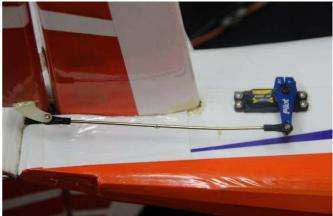
Locate and cut the covering where the servo will be installed, at the rear of the fuselage, under the elevator.
