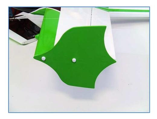
Finalize the installation of the wing deflectors with the screws provided with the Kit
