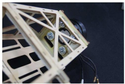
Place the cowl on the model and measure the gap between the firewall and motor hub/spinner position.
