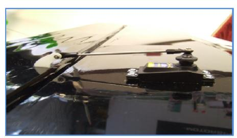
Locate and cut the covering where the servos will be installed.
