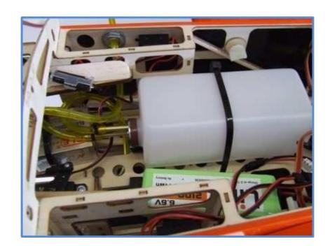
After engine installation, then install the ancillary components such as ignition battery, fuel tank, receiver, etc...
