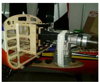
When you finished hole drilling, Install the the plastic support to the fuselage, use the mounting screws to tightening it.
