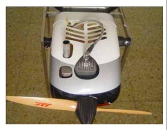
YAK-54 73" need an extension tool with a proper size ball driver and handle by cutting standard ball driver in half .Some small heat shrink tubing are attached to the ball driver to hold in place. You have to reattach the cowl in the future by this method
