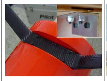
2. Install the landing gear axles with lock nut, but do not tighten
