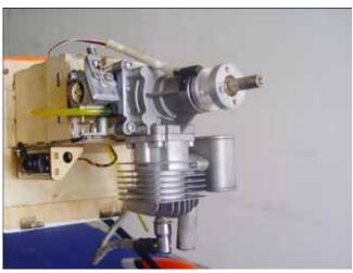
Remember: Use Bue Loctite on all engine mounting screws
