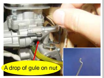
2. Determine where the throttle servo mounting tray is going to be mounted on the engine box to get the straight and precise throttle linkage connection. Then make a mark and epoxy the tray in place .Finally secure with self-tapping screws
