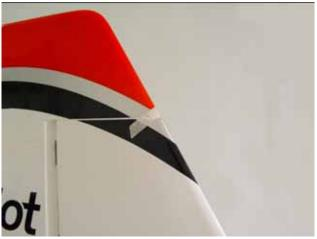
3. Attach the pre-installed boll link to the rudder horn and not tighten the locking nut
