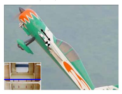
Your balance at the CG will determine batteries final mounting location .Mount batteries and secure with Nylon ties
