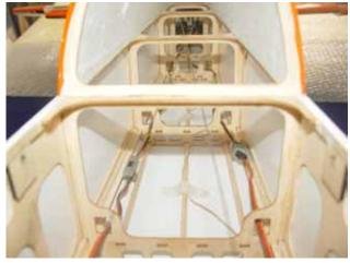
3. Install servos with mounting screws. Face the brand toward the rear of fuse. Use 1mm bit to drill the mounting holes
