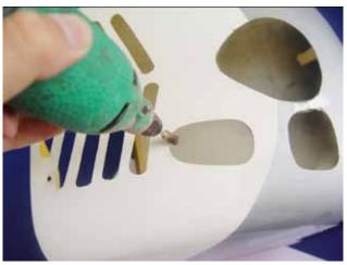
3. Also cut out for clearance for the exhaust pipes
