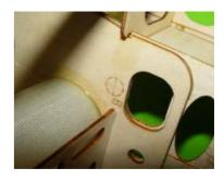
The location of CG has been marked inside plane as show. Usually it is near the wing tube.
