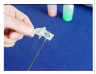
5. Slide the horn into slot slightly and Mount the locking plate in place. Wipe away excess epoxy with rubbing alcohol
