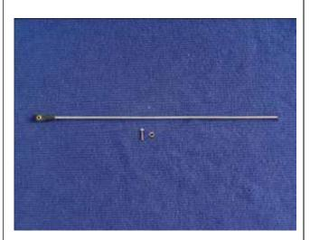
1. Install the engine throttle arm witn a little Blue Loctite. Measure and cut the extra wire .Then bend to a sharp of "z" as shown. Mount the throttle pushrod to engine
